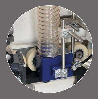
The application unit is connected to the existing machine exhaust. The switching and workpiece detection is carried out via the known RIEPE® electronics or via integration into the machines PLC by your machine manufacturer.
